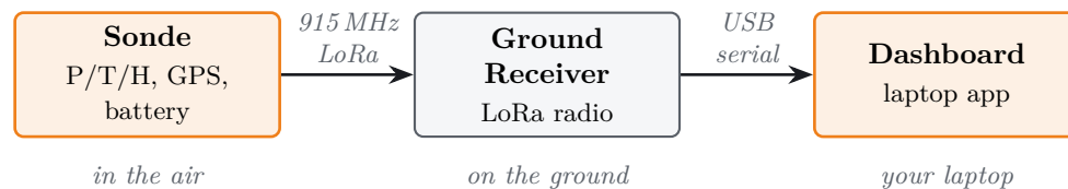
Figure 1.1: The PTH Sonde signal chain: the airborne sonde transmits telemetry over LoRa to a ground receiver, which forwards it over USB to the desktop dashboard.
