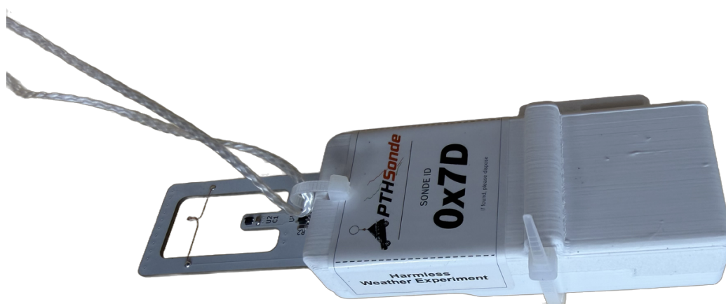
Figure 3.3: The finished sonde tied onto the flight line, ready to be attached below the parachute and balloon. Note the exposed thermistor board (left) that reads the true air temperature.
