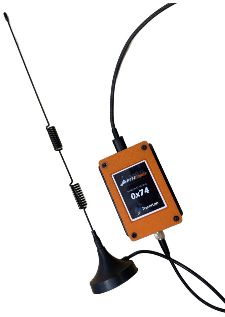
Figure 4.1: The ground station: the receiver box (here Ground Station 0x74 ), its magnetic-mount 915 MHz whip antenna, and the USB lead to the laptop.
