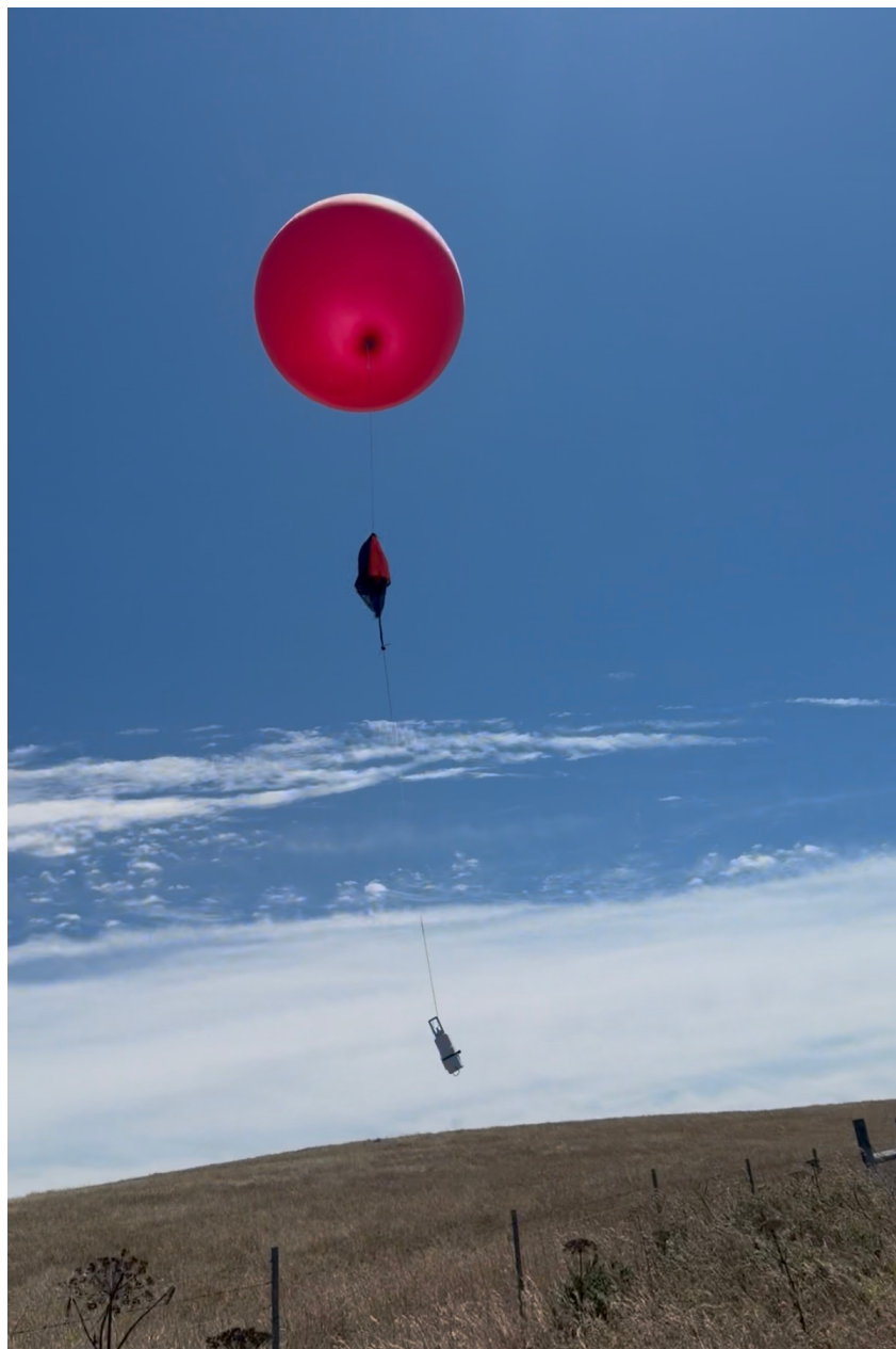
Figure 6.1: Release. Let the balloon lift the flight line and payload cleanly out of your hands; the dashboard should immediately show the climb rate go positive.
