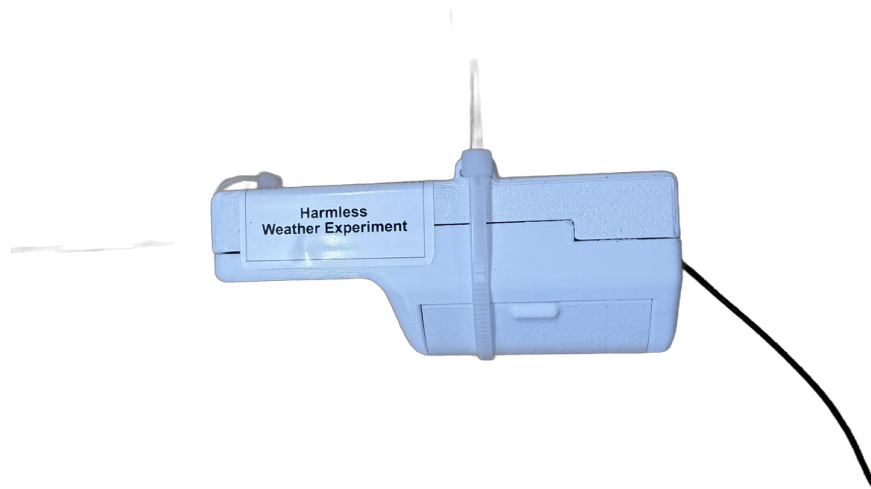
Figure 3.2: The closed enclosure with the outer door zip-tied shut. The printed sticker carries the sonde's hex ID and the finder instructions.
