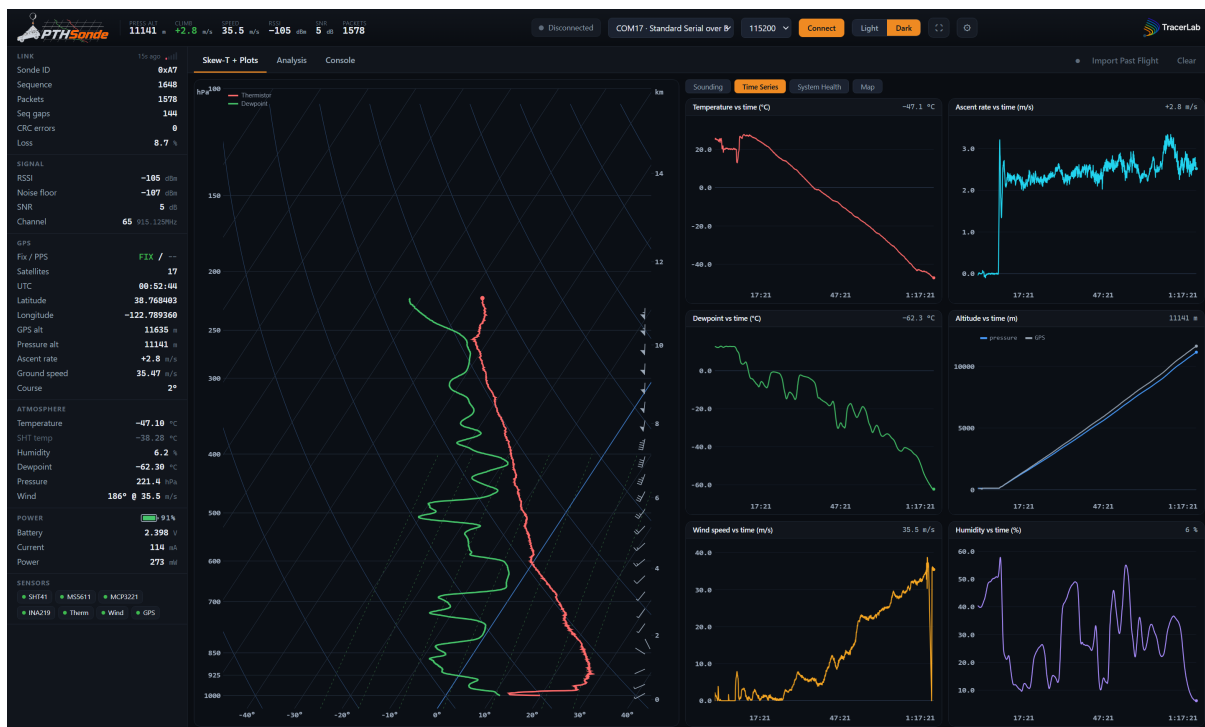
Figure 4.4: Time Series view — every channel plotted against time for a quick sanity check of the whole flight.
