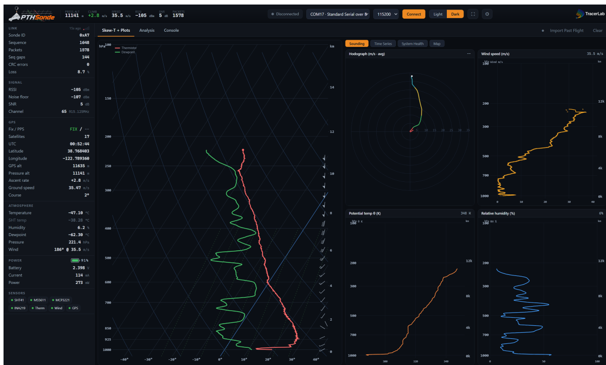
Figure 4.2: The live dashboard during a flight. Left: link, signal, GPS, atmosphere, power and per-sensor health. Centre: the Skew-T with the thermistor (red) and dewpoint (green) traces and wind barbs. Right: hodograph, wind-speed, potential-temperature and relative-humidity profiles.
